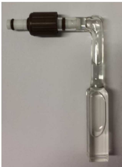
Figure S1. 10 mm pathlength quartz cell fused with a J-Young valve used for luminescence data collection of air sensitive compounds.
