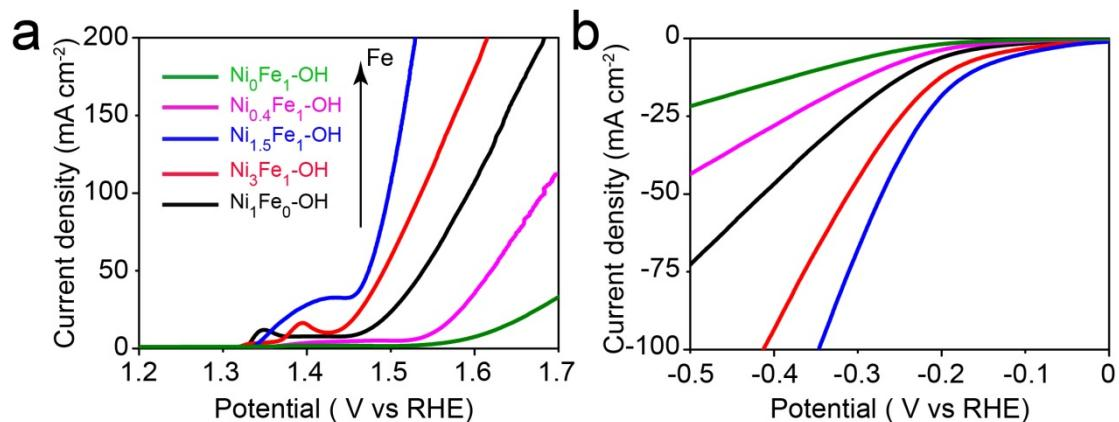
**Figure S11.** LSV curves for samples with varying Fe content toward (a) OER and (b) HER reactions, from which it could be drawn that  $\text{Ni}_{1.5}\text{Fe}$  was optimal.
