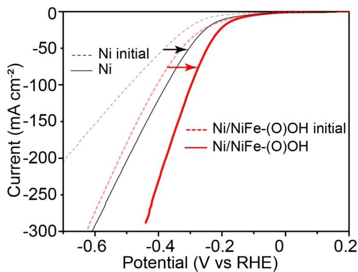
**Figure S9.** HER LSV curves of the Ni/NiFe (oxy)hydroxide before and after oxidation treatment, showing that the HER performance was to some extent optimized by the gentle oxidation treatment.
