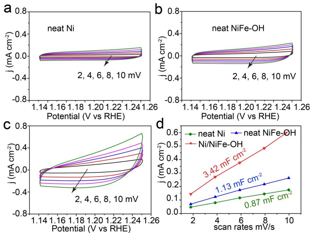
**Figure S14.** (a-c) Cyclic voltammograms curves measured in a non-Faradaic region (1.14-1.25 V) at varying scan rates, 2, 4, 6, 8, 10  $\text{mV s}^{-1}$  for the Ni/NiFe heterostructure nanotube, neat Ni, and neat NiFe (oxy)hydroxide. (d) Estimation of electrochemical double-layer capacitances for the samples. The designed Ni/NiFe nanotube manifested the largest value, underlining the advantage of the designed structure.
