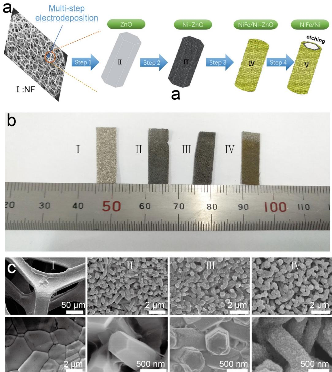
**Figure S1.** (a) Schematic diagram for sample growth, (b) digital photographs, and (c) low-magnification SEM images for samples at the different growth steps. The color change evidenced the successive growth of Zn, Ni, and NiFe (oxy)hydroxide.
