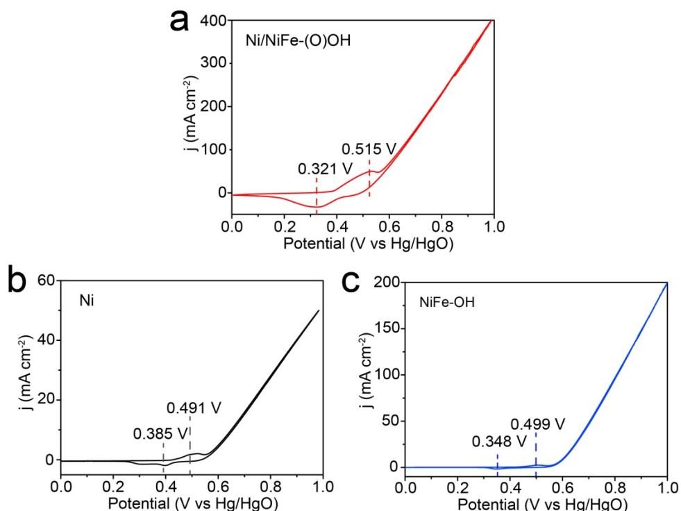
**Figure S16.** CV curves for the (a) Ni/NiFe (oxy)hydroxide heterostructure compared with (b,c) the individual components.
