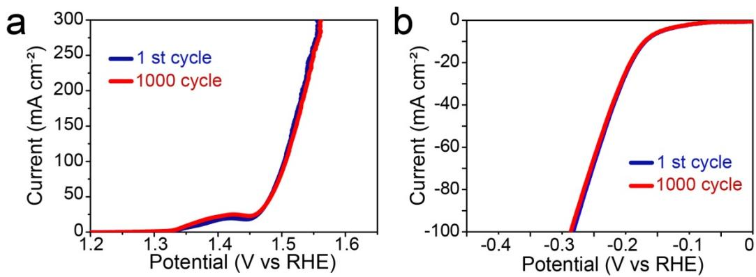
**Figure S12.** LSV curve comparison for (a) OER and (b) HER cyclic reactions.
