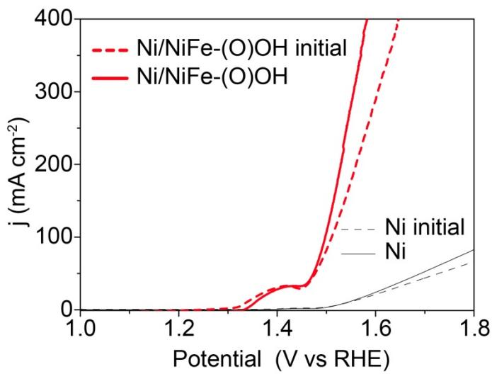
**Figure S10.** OER LSV curves of the Ni/NiFe (oxy)hydroxide before and after oxidation treatment, showing that the performance was little affected.
