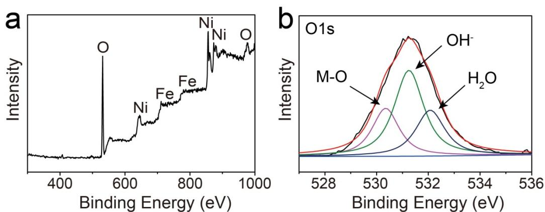
**Figure S8.** (a) XPS full-range and (b) O1s spectra for Ni/NiFe (oxy)hydroxide nanotubes.
