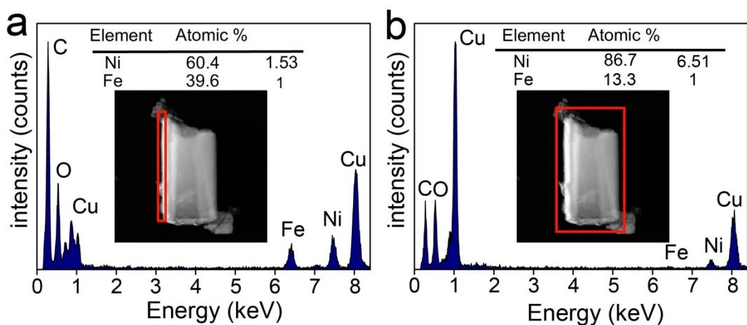
**Figure S6.** EDS spectrum for (a) outer NiFe (oxy)hydroxide and (b) the whole wall.
