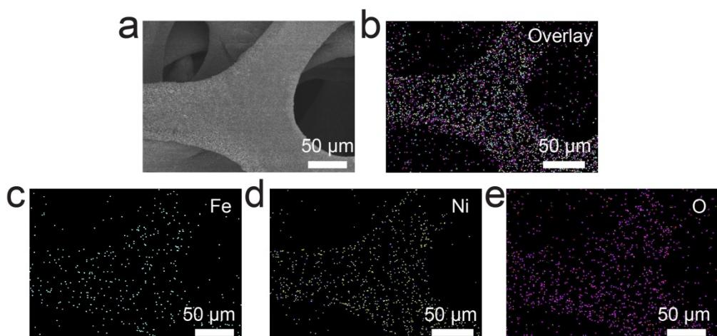
**Figure S5.** (a) Low-magnification SEM image for the final product of Ni/NiFe (oxy)hydroxide nanotube arrays and corresponding elemental mapping images of (b) overlaying, and individual (c) Fe, (d) Ni, (e) O elements, showing homogeneous distribution for all elements, which implied even growth of the product.
