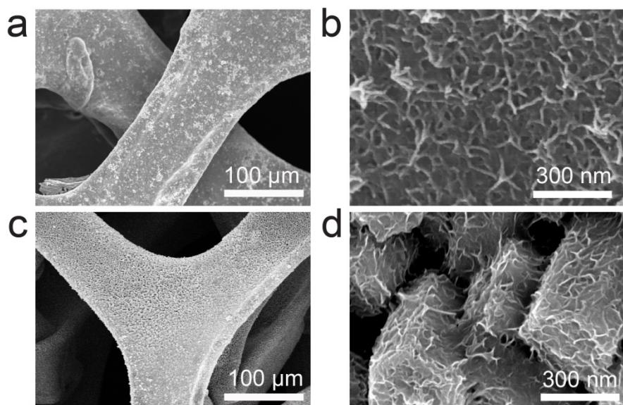
**Figure S7.** NiFe (oxy)hydroxide directly grown on (a-b) Ni foam and (c-d) ZnO. The morphology was sheet-like wrapping on Ni substrate or ZnO rods.
