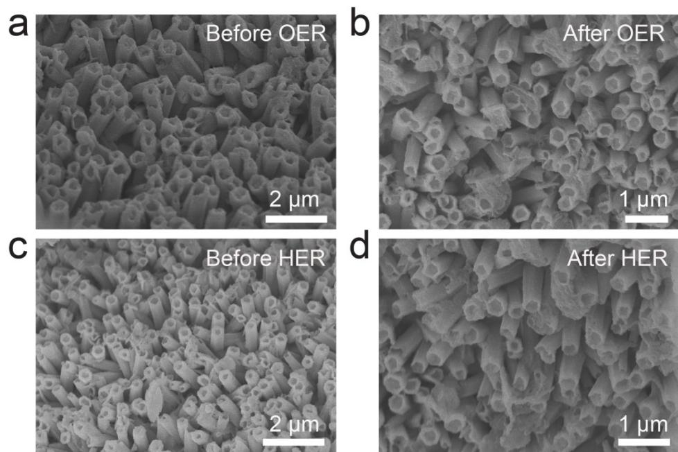
**Figure S13.** SEM morphology comparison before and after (a-b) OER and (c-d) HER cyclic reactions.
