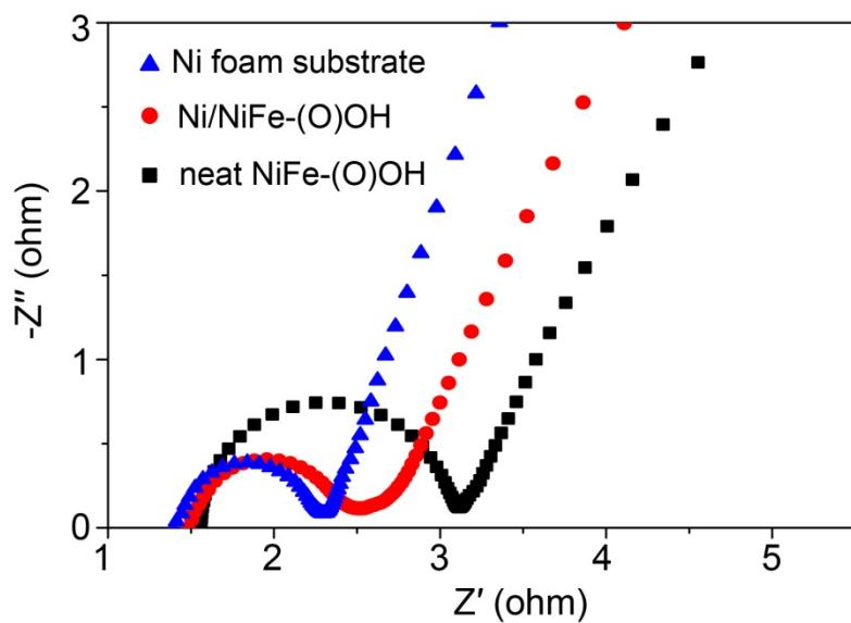
**Figure S15.** Nyquist plots of the samples, which indicated that the Ni seeds could work as effective electron highways for Ni/NiFe heterostructure, displaying electron conductivity even comparable to Ni foam substrate
