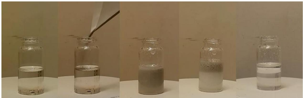
**Figure S2.** Experimental photographs of adding Mg powders to CO<sub>2</sub>-saturated hydrazine hydrate solution for validation of Equation 2. The fundamental of Equation 2 is  $2\text{NH}_2\text{NH}_3^+ + \text{H}_2\text{O} + \text{Mg} \rightarrow \text{Mg}^{2+} + 2\text{NH}_2\text{NH}_2 + \text{H}_2\text{O} + \text{H}_2 \uparrow$ . Similar with ammonium ion, adding water to this system could help generate more hydrogen ions through hydrolysis, thus promote the reaction of Equation 2.
