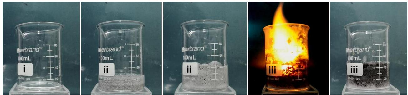
**Figure S1.** Experimental photographs of combustion pyrolysis conversion of CO<sub>2</sub> to NCF sample. (i) Chemical sorption of CO<sub>2</sub>. (ii) Dissolution of the added Mg powders for the formation of homogeneous organic salt of magnesium. (iii) Generation of NCF under combustion pyrolysis reaction and the following acid etching treatment to remove impurities.
