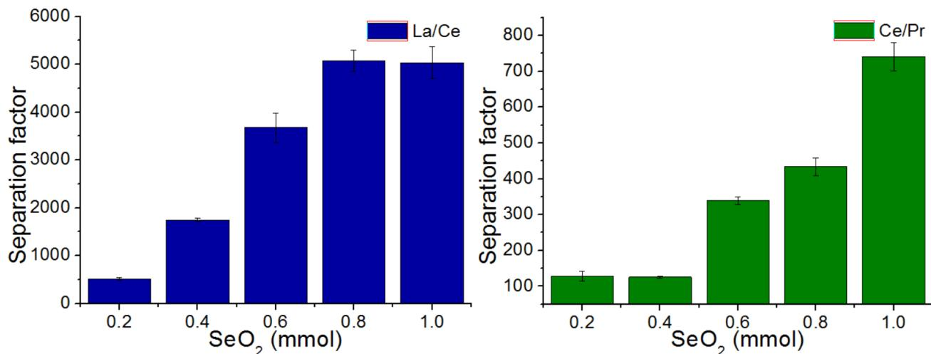
**Figure S11.** Separation factors for binary La/Ce and Ce/Pr under different amounts of  $\text{SeO}_2$ .
