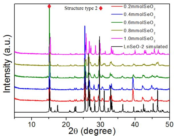
**Figure S7.** Simulated PXRD pattern for **LnSeO-2** and experimental PXRD patterns for **La/Ce** solid products at different reaction conditions (the reactant of  $\text{SeO}_2$ : 0.2 mmol, 0.4 mmol, 0.6 mmol, 0.8 mmol, or 1.0 mmol).
