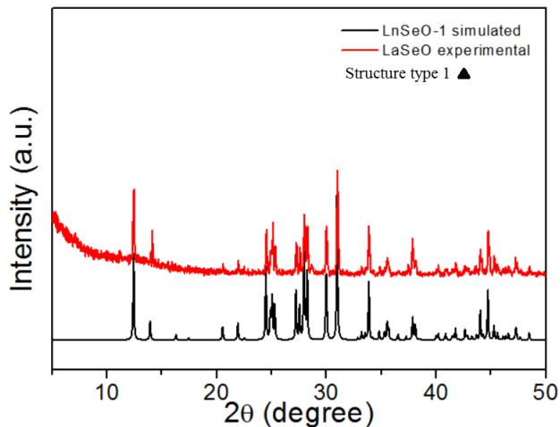
**Figure S1.** Simulated PXRD pattern for **LnSeO-1** and experimental PXRD pattern for LaSeO solid product.
