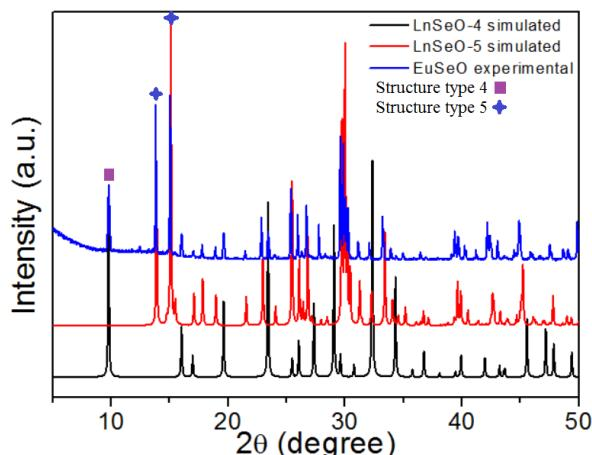
**Figure S4.** Simulated PXRD patterns for **LnSeO-4**, **LnSeO-5** and experimental PXRD pattern for EuSeO solid product.
