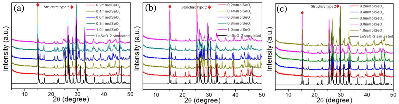
**Figure S9.** Simulated PXRD pattern for **LnSeO-2** and experimental PXRD patterns for (a) Th/La (b) Th/Eu (c) Th/Yb solid products at different reaction conditions (the reactant of  $\text{SeO}_2$ : 0.2 mmol, 0.4 mmol, 0.6 mmol, 0.8 mmol, 1.0 mmol).
