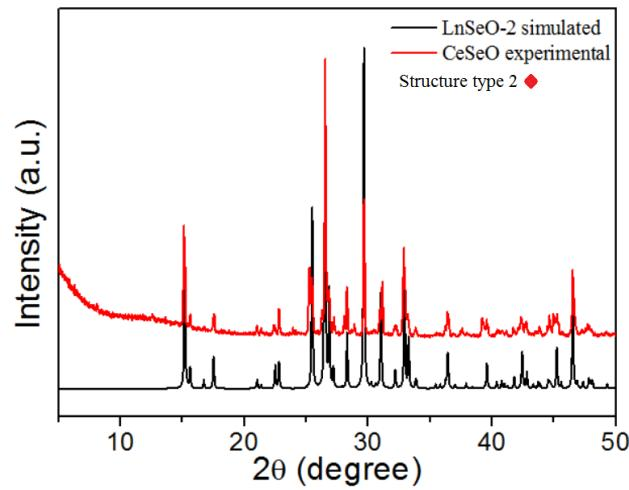
**Figure S2.** Simulated PXRD pattern for **LnSeO-2** and experimental PXRD pattern for CeSeO solid product.
