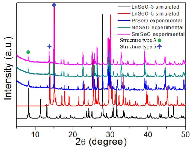
**Figure S3.** Simulated PXRD patterns for **LnSeO-3**, **LnSeO-5** and experimental PXRD patterns for LnSeO ( $\text{Ln} = \text{Pr}$ ,  $\text{Nd}$ , and  $\text{Sm}$ ) solid products.
