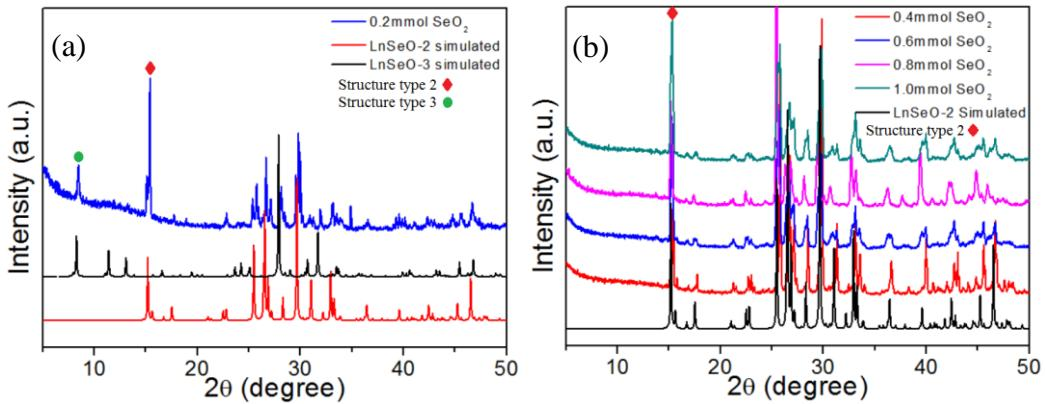
**Figure S8.** Simulated PXRD pattern for **LnSeO-2** and experimental PXRD patterns for Ce/Pr solid products at different reaction conditions (the reactant of  $\text{SeO}_2$ : 0.2 mmol, 0.4 mmol, 0.6 mmol, 0.8 mmol, or 1.0 mmol).
