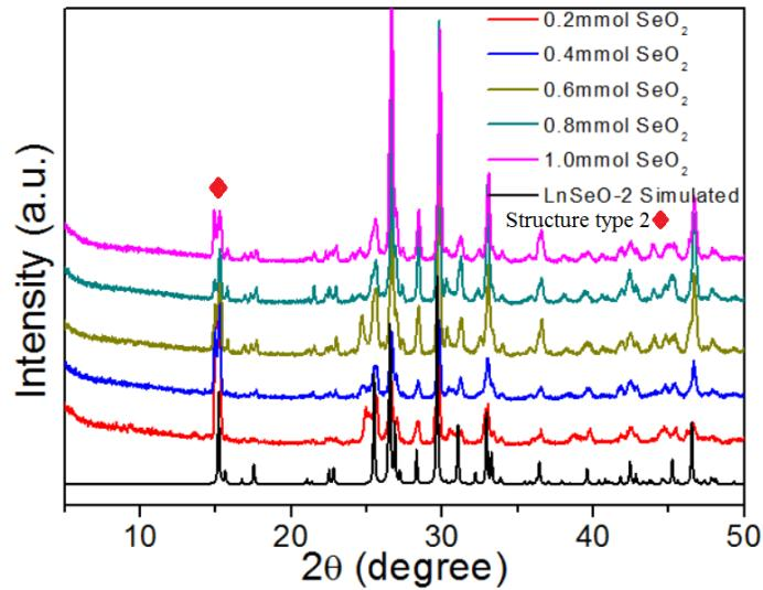
**Figure S10.** Simulated PXRD pattern for **LnSeO-2** and experimental PXRD patterns for  $\text{Th}^{4+}/\text{Ce}^{4+}$ /simulated monazite solid products at different reaction conditions (the reactant of  $\text{SeO}_2$ : 0.2 mmol, 0.4 mmol, 0.6 mmol, 0.8 mmol, or 1.0 mmol).
