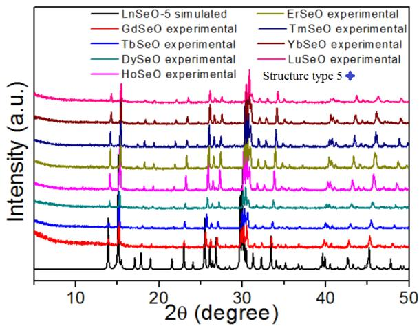
**Figure S5.** Simulated PXRD pattern for **LnSeO-5** and experimental PXRD patterns for **LnSeO** ( $\text{Ln} = \text{Gd}, \text{Tb}, \text{Dy}, \text{Ho}, \text{Er}, \text{Tm}, \text{Yb}$ , and  $\text{Lu}$ ) solid products.
