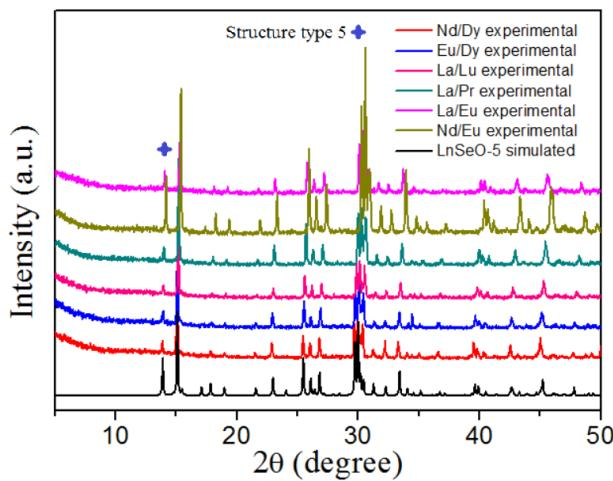
**Figure S6.** Simulated PXRD pattern for **LnSeO-5** and binary  $\text{Nd}/\text{Dy}$ ,  $\text{Eu}/\text{Dy}$ ,  $\text{La}/\text{Lu}$ ,  $\text{La}/\text{Pr}$ ,  $\text{La}/\text{Eu}$ ,  $\text{Nd}/\text{Eu}$  experimental PXRD patterns.
