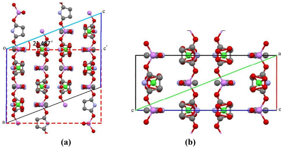
Figure S4 the unit cell unit cell length and  $\beta$  angles for (a) 1-LTP and (b) 1-RTP
