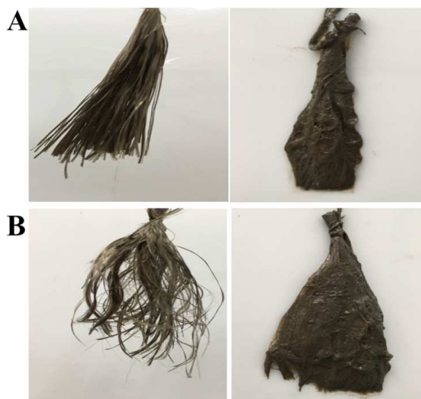
Figure S2 Pictures of BF (A) and MBF (B) before and after microorganism immobilization tests
