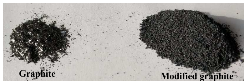
Figure S2 Photographs of graphite and modified graphite. After microwave treating, the volume of graphite increased.
