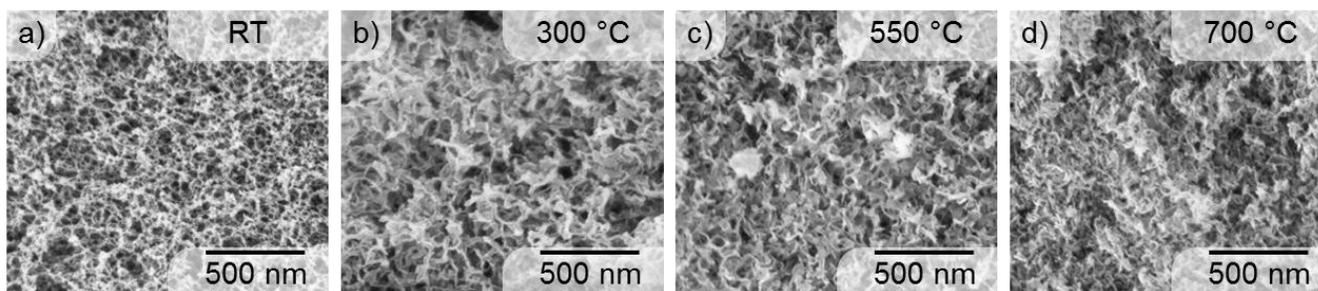
Figure S1: SEM images of sheet-like morphology of alumina aerogels which retained after each heat treatment. a) room temperature (RT), b) 300 °C, c) 550 °C, d) 700 °C
