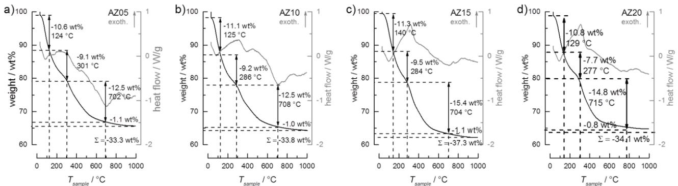
Figure S11: DTA-TG measurements of alumina mixed with zirconia (AZ) aerogels; Ordered by increasing zirconium content in at% Zr, a) 5 at% Zr AZ05, b) 10 at% Zr AZ10, c) 15 at% Zr AZ15, d) 20 at% Zr AZ20. While temperature of second step is decreasing the DTA signal is increasing in reason of earlier organic decomposition of zirconia.
