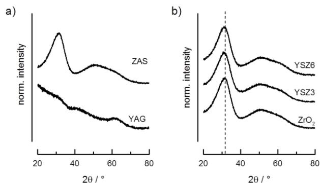
Figure S8: XRD patterns of amorphous mixed aerogels; a) yttrium aluminum garnet (YAG) and zinc aluminum spinel, as well as b) zirconia yttrium stabilized zirconium oxide 3 at% Y (YSZ<sub>3</sub>), yttrium stabilized zirconium oxide 6 at% Y (YSZ<sub>6</sub>) which show a slightly shift of reflections to lower angles due to a lattice contraction.
