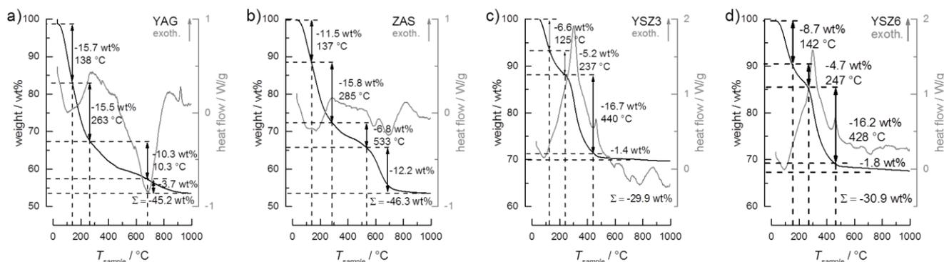
Figure S7: DTA-TG measurements of mixed aerogels; a) yttrium aluminum garnet (YAG), b) zinc aluminum spinel, c) yttrium stabilized zirconium oxide 3 at% Y (YSZ<sub>3</sub>), d) yttrium stabilized zirconium oxide 6 at% Y (YSZ<sub>6</sub>)
