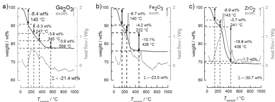
Figure S4: DTA-TG measurements of a) gallia, b) iron oxide and c) zirconia aerogels
