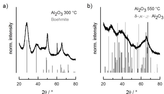
Figure S2: XRD of alumina aerogels annealed a) at 300 °C with (pseudo-)boehmite structure and b) at 700 °C with mixed aluminum oxide structure.
