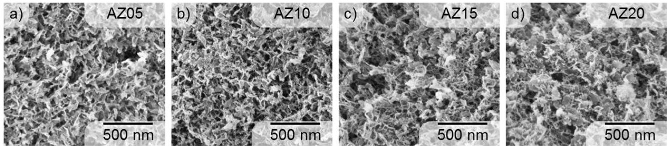
Figure S9: SEM images after annealing at 300 °C. Sponge-like morphology occurs increasingly due to Zr content from 0 to 20 at% Zr. Ordered by increasing zirconium content in at% Zr, a) 5 at% Zr AZ05, b) 10 at% Zr AZ10, c) 15 at% Zr AZ15, d) 20 at% Zr AZ20.
