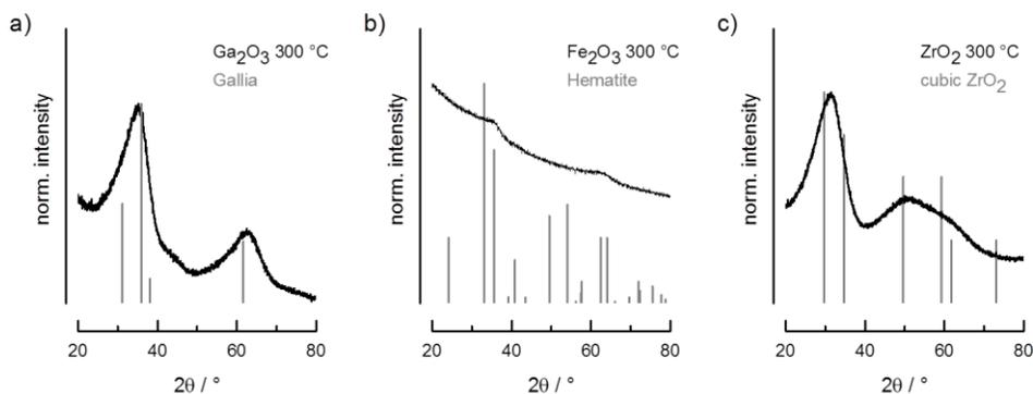
Figure S5: XRD patterns of mainly amorphous of a) gallia, b) iron oxide and c) zirconia aerogels.
