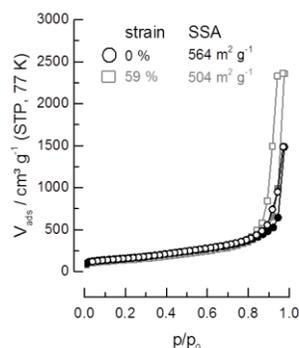
Figure S3: 81 points isotherms of alumina aerogels annealed at 300 °C before and after pressure test (strain 59 %). The porous networks represent a mixture of type II and IV isotherm. Both isotherms show a similar curve shape, but adsorbed volume after densification is increased due to the compression of former large macropores and since that are accessible for the nitrogen physisorption. Hence, network structure retained intact after compression.
