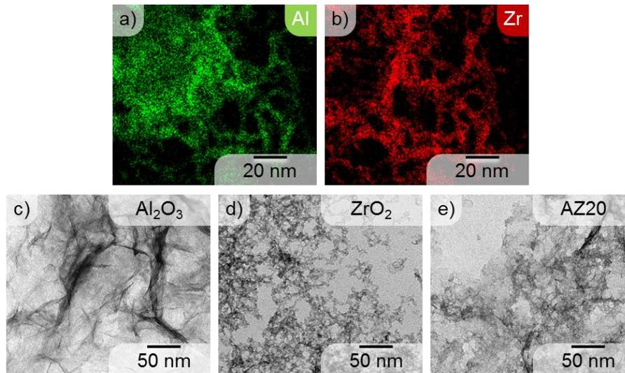
Figure S10: a) Aluminum and b) zirconium distributions for the field of view shown in figure 6. Bright-field TEM images of c) pure alumina aerogel, d) pure zirconia aerogel and e) AZ20 aerogel after annealing at 300 °C
