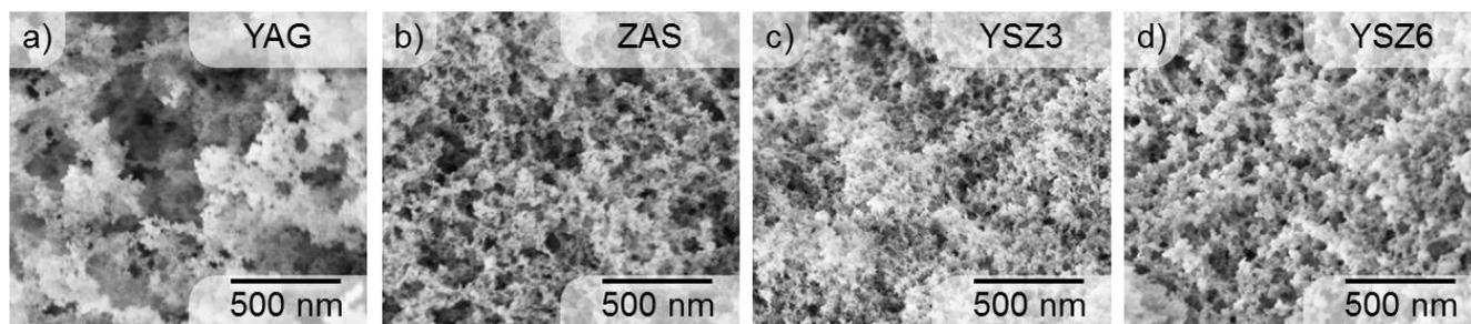
Figure S6: SEM images of mixed aerogels after annealing at 300 °C; a) yttrium aluminum garnet (YAG), b) zinc aluminum spinel, c) yttrium stabilized zirconium oxide 3 at% Y (YSZ<sub>3</sub>), d) yttrium stabilized zirconium oxide 6 at% Y (YSZ<sub>6</sub>)
