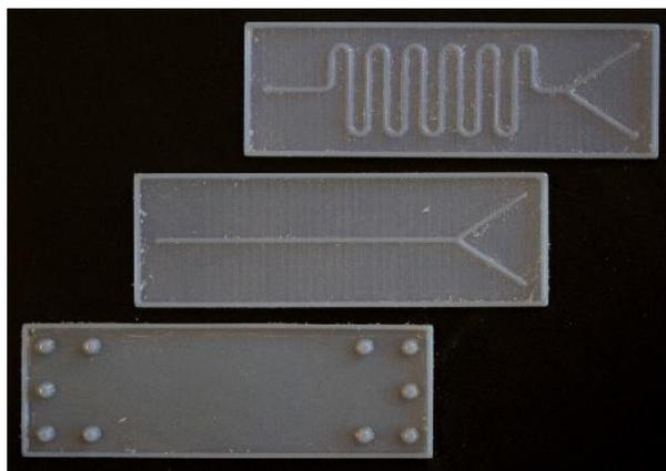
**Figure B10:** 3D printed molds for PDMS casting: bottom part (serpentine channel or Y channel) and top part (below).
