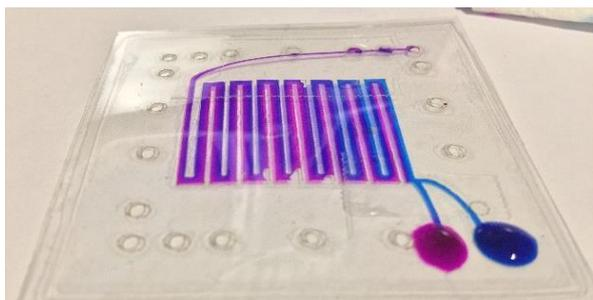
**Figure B7:** Example of large 50 x 50 mm foil chip design (laser-cut serpentine mixer, 300  $\mu\text{m}$  channel width) filled with dyed water. The additional holes are in the (universal) top layer allow modification of the channel pattern using scissor or knife before assembly.
