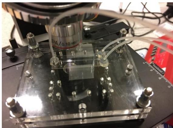
**Figure B5:** Assembled chip PMMA holder holding an 15 x 45 mm Y reactor foil chip (the channel of which was enlarged to 0.3 mm by scissors before assembly) and connected to the tubing using silicon ferrules. With this experiment a Calcite precipitate is formed from 0.025 M CaCl<sub>2</sub> and 0.1 M NaHCO<sub>3</sub> (for details see figure 7 of the main article). The reaction is observed using the 40x magnification of a standard microscope.
