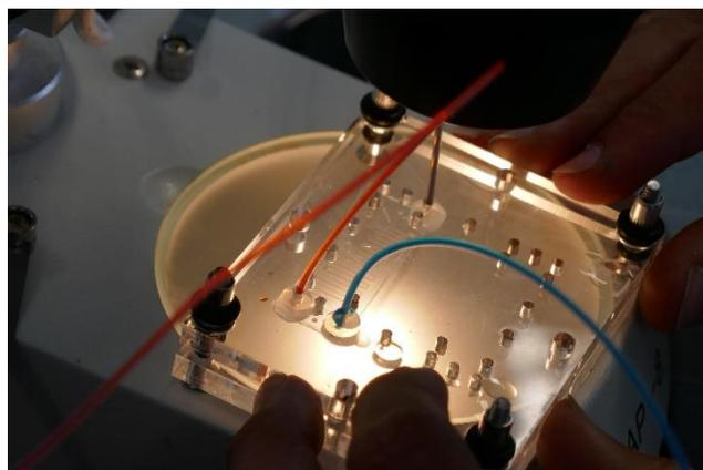
**Figure B6:** PMMA holder in an experiment with a 3-inlet serpentine mixer (of which 2 inlets were closed with adhesive tape), used with dyed water to study the mixing properties of the chip. In this case a binocular microscope is used to study the reaction.
