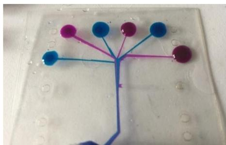
**Figure B8:** A 50 x 50 mm chip, with laser-cut entrance holes and scissor-cut channels, filled with dyed water after assembly. See figure 6 in the main article for details. The chip will fit the PMMA holder.
