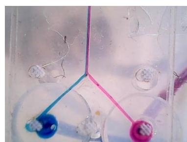
**Figure B4:** Silicon ferrules connect the H-reactor in the PMMA holder. Note the dashed alignment indicators in the bottom plate.
