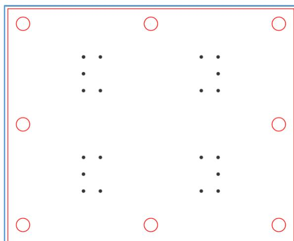
**Figure B2A:** Design of PMMA chipholder bottom plate, with engraved spots for alignment of the fluidic connections. The holder is produced from cast PMMA of 6 mm thickness using the Trotec Speedy 300 laser cutter. Cutting is done at 500 dpi, 10,000 Hz, power 100, speed 0.3. Engraving of dots: 500 dpi, 10,000 Hz, power 100, speed 3.
