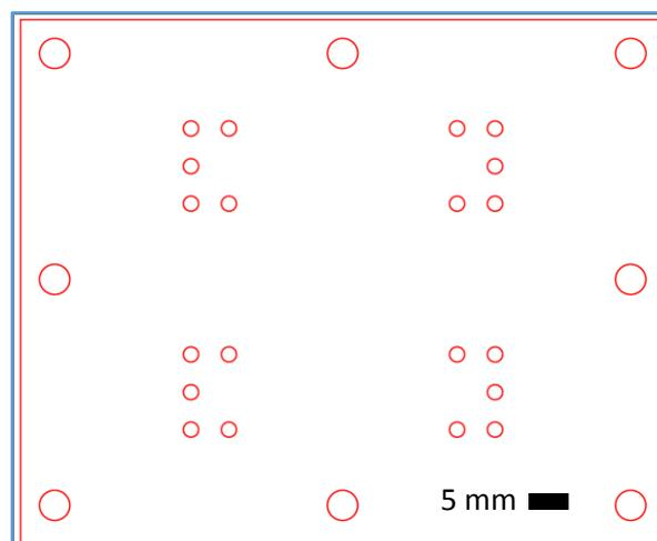
**Figure B2B:** Design of PMMA chipholder top plate, with 2 mm holes (for tubing) and 4 mm (for screws). Bar indicates 5 mm. (A similar plate, with 3.4 mm holes, made from 2 mm PMMA is added between the chip and the top plate to fit perlast ferrules with stainless steel ring). A smaller variety of the chip holder holds only one 15 x 45 mm chip. Bar indicates 5 mm.
