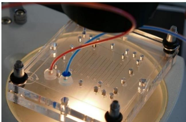
**Figure B9:** The PMMA holder in an experiment with the 50 x 50 mm serpentine mixer, mounted using silicon ferrules.
