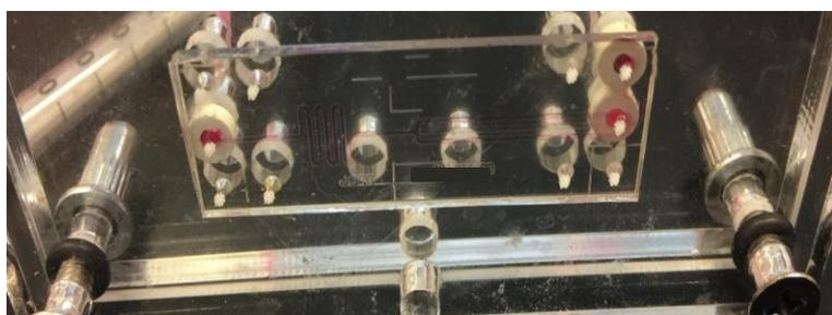
**Figure B3:** Detail of the PMMA holder holding the FFDG droplet generator. For this experiment, Perlast ferrules and an adapter plate (2 mm thickness, with 3.4 mm holes to fit the SS ferrule rings placed directly below the top plate) were used.
