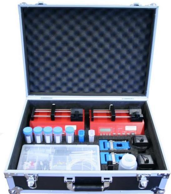
*Figure A1: One of the practical kits containing the equipment for Lab-on-a-chip experiments in the classroom.*
